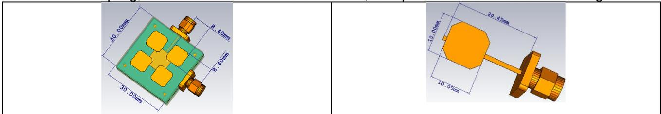
Figure 1. Antenna & the Feeding structures; Antenna patches (left), antenna feeding network (right)
